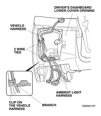
11. Route the ambient light harness under the dashboard toward the center console, and attach the ambient light harness clip to the hole in the vehicle frame.
