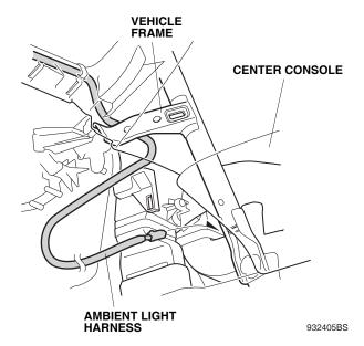
15. Route the ambient light harness through the center console towards the passenger's side of the vehicle. Using one wire tie, secure the ambient light harness to the vehicle frame.
