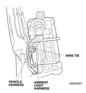
**Installing the Ambient Lights**
