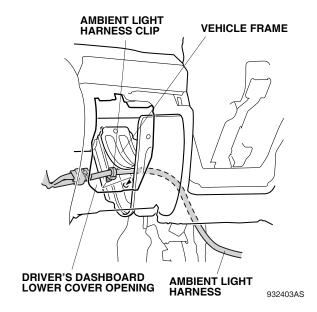
12. Attach the other ambient light harness clip to the dashboard tab.
