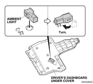
22. Plug the ambient light harness 2-pin connector into the ambient light, and reinstall the driver's dashboard under cover.
