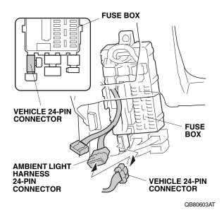
18. Attach the ambient light harness 24-pin connector (just plugged in) to the vehicle 24-pin connector as shown.
