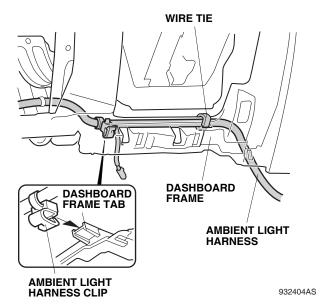
13. Using one wire tie, secure the ambient light harness to the dashboard frame.
