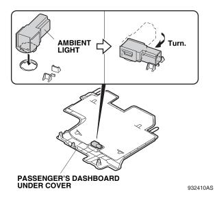
24. Plug the ambient light harness 2-pin connector into the ambient light, and reinstall the passenger's dashboard under cover.
