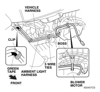
17. At the fuse box, unplug the vehicle 24-pin connector, and plug it into the ambient light harness 24-pin connector.
